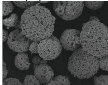
FUJIMI's yttrium oxide powder are spherical particles and designed to achieve the highest deposition efficiency. FUJIMI has sophisticated classification technology and powder size can be customized to suit a wide range of application needs.
